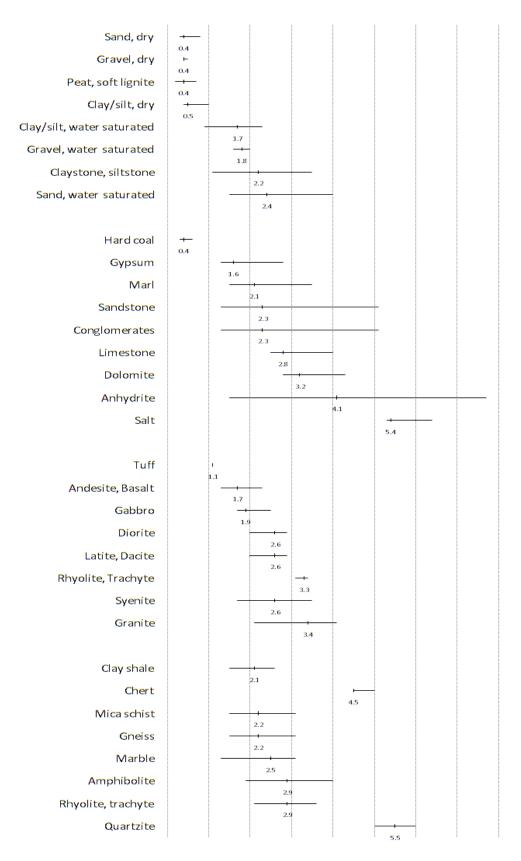
Figure C1: Ranges of thermal conductivity for different rock types, indicating recommended values. The data is the same as that in table B1. Horizontal lines represent the range of thermal conductivity for each rock type. Recommended values are written on the chart.
